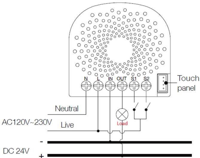
**Note:** The "IN" terminal should be connected to the "-" of 24VDC input.
