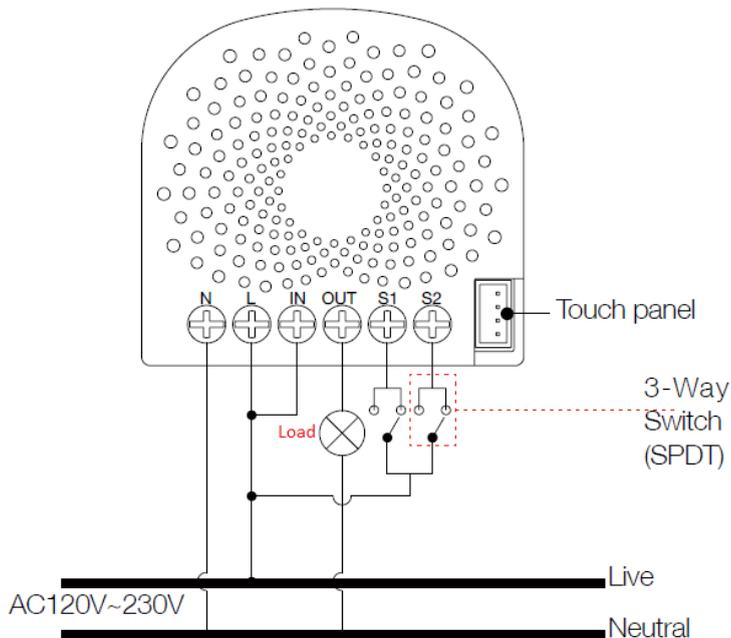
3. Auto-Detect external switches connected.
