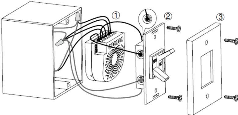
**Note:** 1. The gang box should be sized 3×2×2.75 inch / 75×50×70 mm or larger, minimum volume 14 in / 230cm .
