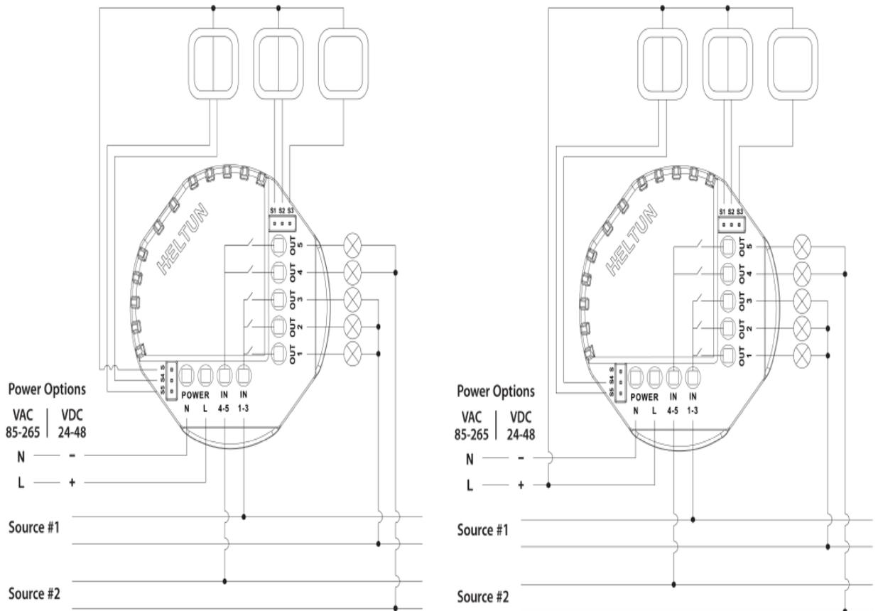
**Figure 2: Power, Loads & External Switches Connection Diagram**
