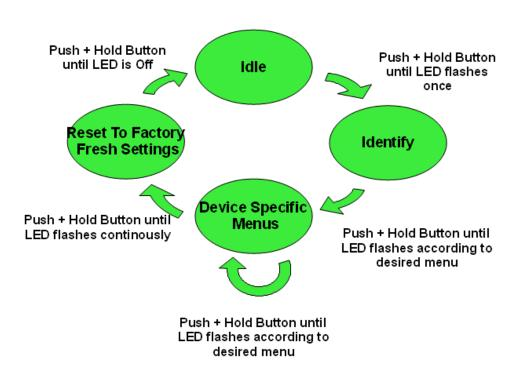
When cycling through the menu modes, the state is indicated by a number of 100ms blinks on the LED. As illustrated in the figure, the menu system allows for device specific modes (e.g. Pair Devices for Devices such as relays and occupancy sensors).
