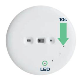
**Remark:** You can also just reset the counters. To do this, all you have to do is insert a pin and click **1 time** into the **"R" hole.**
